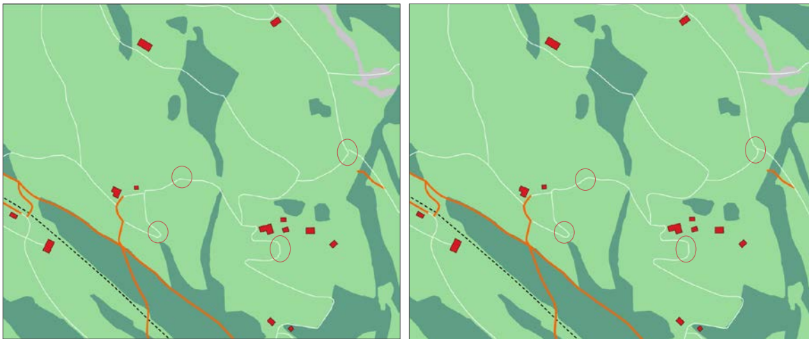
Figure 5: Line to Bezier: plugin to create Bezier curves of the local roads
