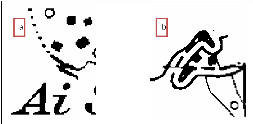
Figure 5: Problems, which occurred during automatic raster cleaning (a- representation of the letter "i"; b- bold lines and the buildings)
