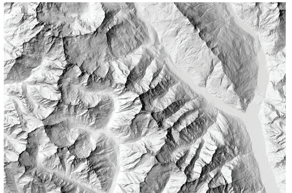
Figure 3: Shaded relief with the aerial perspective effect (Brassel, 1974), calculated within watersheds, and complemented with changes of the light direction
