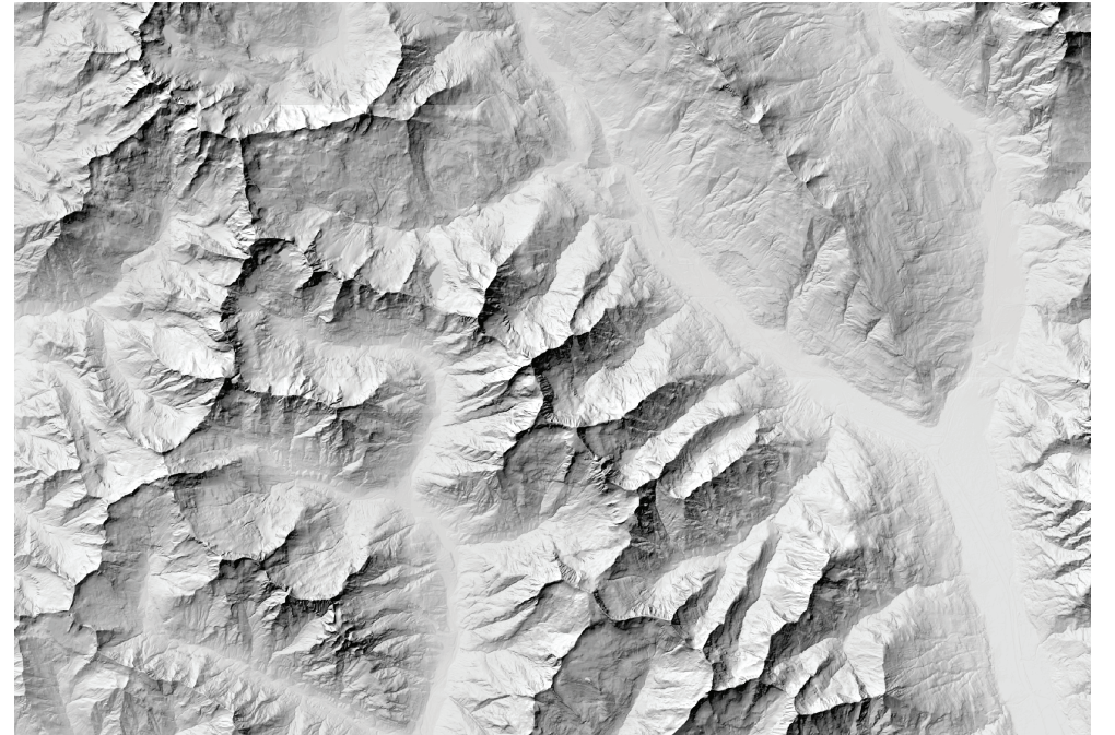
Figure 2: Shaded relief generated using the Hillshade function combined with the aerial perspective effect (Brassel, 1974) calculated within watersheds
